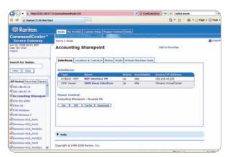
Stay connected to virtual servers even when they are moved from one virtual host to another. Issue on, off, cycle or suspend virtual power commands using the control buttons.
